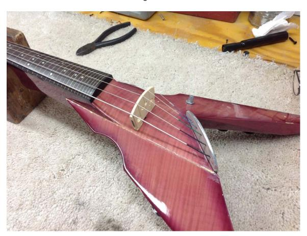
3. Loosen all strings until the bridge can be placed face down. On top of the instrument, place a piece of cloth or paper towel between the bridge and top to prevent scratching.
